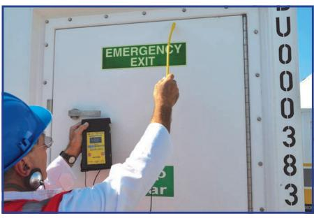
DOOR-SAFE™ is an American Bureau of Shipping (ABS) Type Approved ultrasonic unit that provides a quick and simple method of establishing water and weather tightness in doors, hatches and windows.
